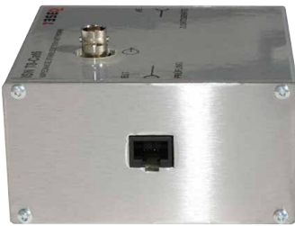
ISN T8-Cat6 with view to the EUT connection RJ45
